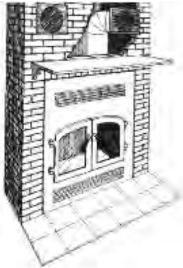
Advanced technology fireplaces combine the decorative flexibility of traditional fireplaces with the clean burning and high efficiency of advanced wood stoves.
