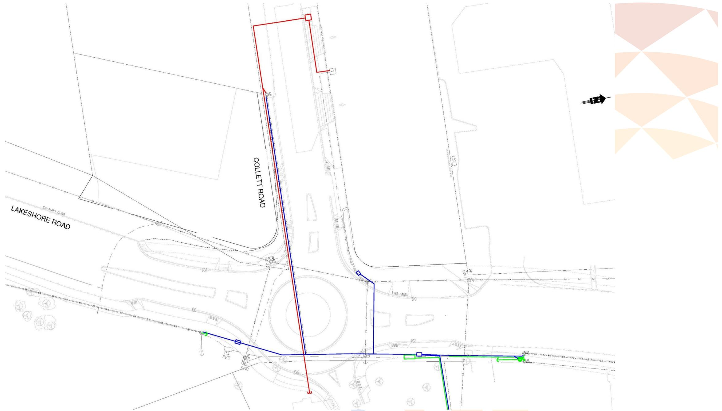
Roundabout geometry requires relocation of existing aerial utilities, and converting aerial wires to underground would result in a safer and cleaner-looking intersection.
