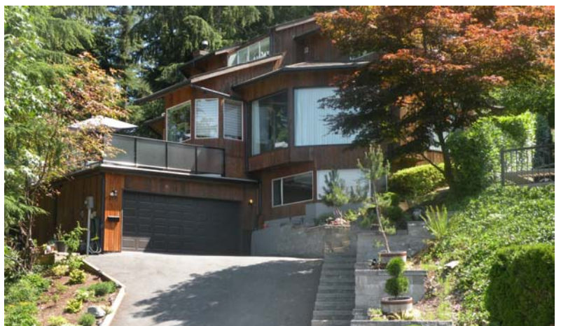
House stepping up hill parallel to slope, roof line matches terrain
