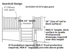
Cable guards (horizontal and vertical) NOT permitted in the City of Kelowna. Guards MUST BE non climbable. No permanent fixtures allowed adjascent to guards (ie benches). IF deck surface to grade is UNDER 4.2 metres, structural horizontal guards allowed. Consult with Building Inspector.
