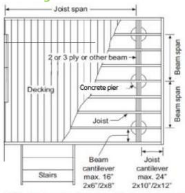
NOTE: Maximum cantilevers apply when joists carry uniform distributed roof loads. Other point loads to transfer directly to the foundation.
