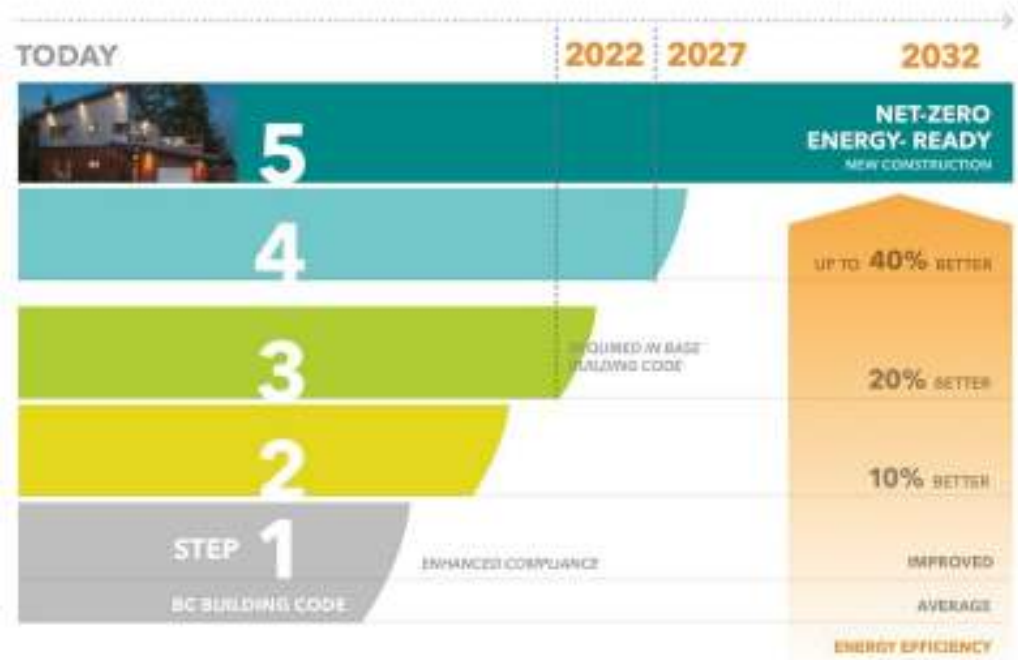
FIGURE 1: THE FIVE PERFORMANCE STEPS OF THE BC ENERGY STEP CODE (PART 9 BUILDINGS)
