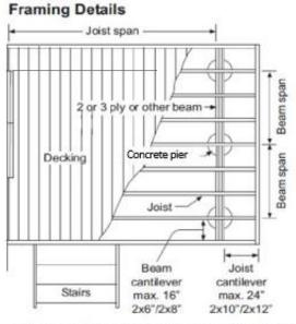
NOTE: Maximum cantilevers apply when joists carry uniform distributed roof loads. Other point loads to transfer directly to the foundation.
