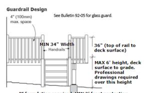
IF foundation required, MIN 2' frost protection required, MIN 6" exposed concrete above grade
